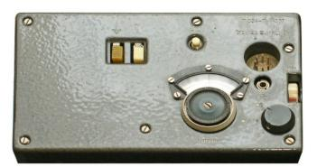
Prototype or earlier version of the Merkur receiver with project number TI 534-P, used with the Sirius III. The tuning graph of the receiver in this picture is missing. See also the Sirius III in Chapter 9.
